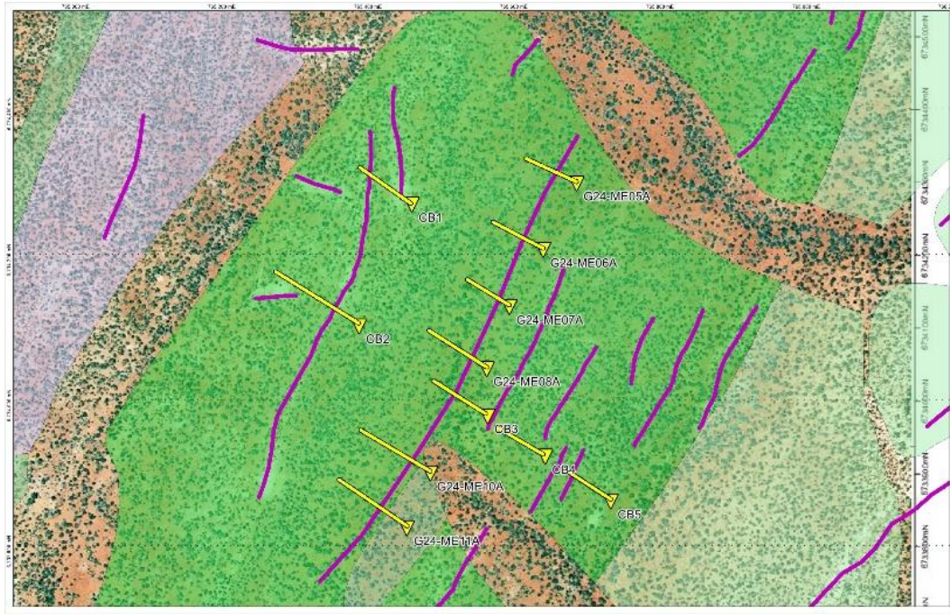
Figure 17 Proposed drilling as a section across multiple dykes, and along strike to determine lateral fractionation.
